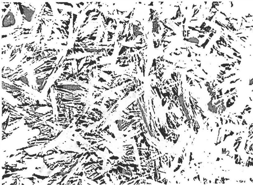
Fig. 4.8 Photomicrographs showing the typical microstructure of sinter containing 40% specularite and 2% quick-lime a) lath shaped and blocky Ca-ferrite b) acicular Ca-ferrite
