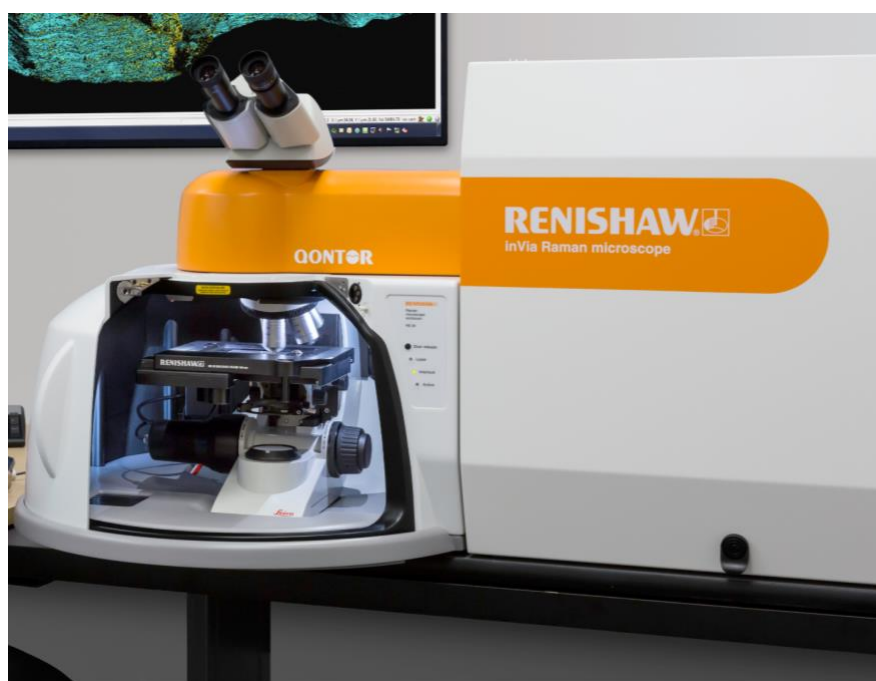
Figure 3.1 Confocal Raman Microscope (Adapted from [62])
