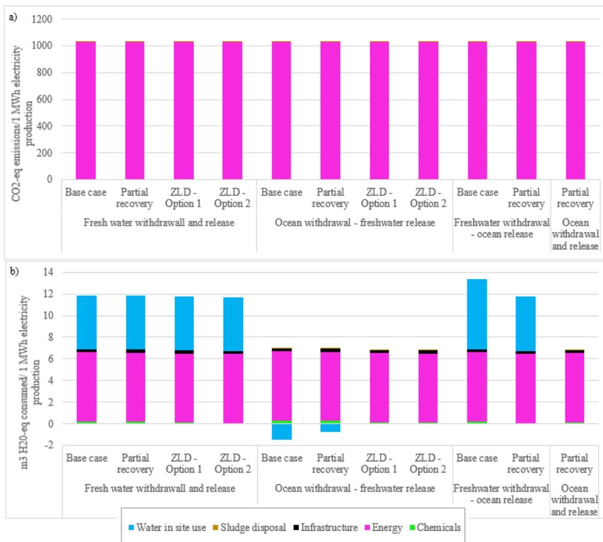
Figure D.3 Different scenarios performance presented in a) for CO 2 -eq emissions and b) for AWARE profile when changing water type for 1 MWh electricity production in French context.
