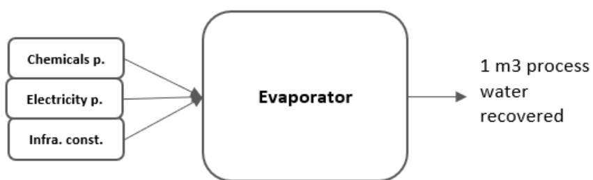
Figure A.8 Evaporator process unit system
