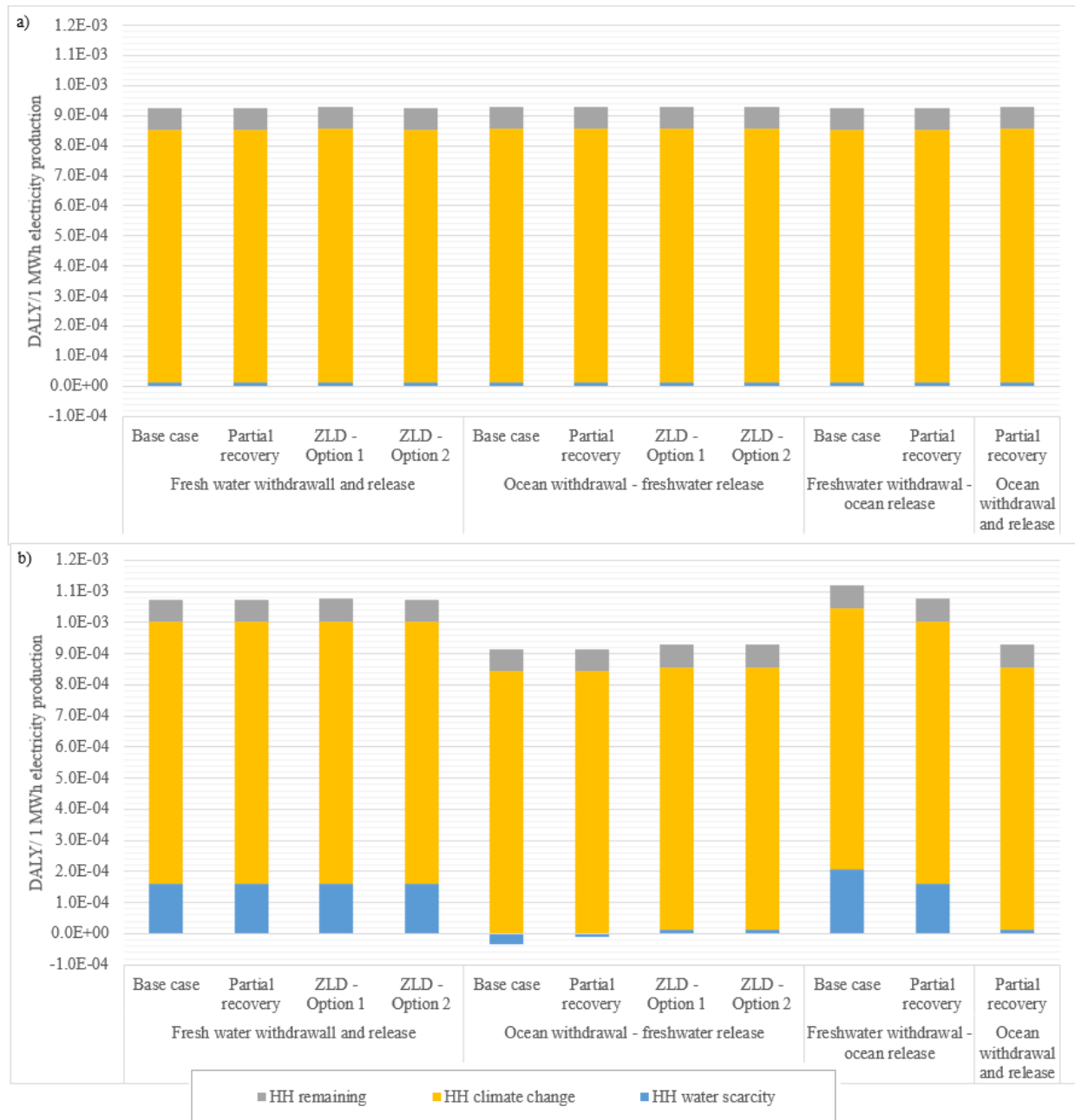
Figure D.4 Human Health impact for 1 MWh electricity production in a) non-scarce or developed countries and b) for non-developed and water scarce place using Algeria as example.
