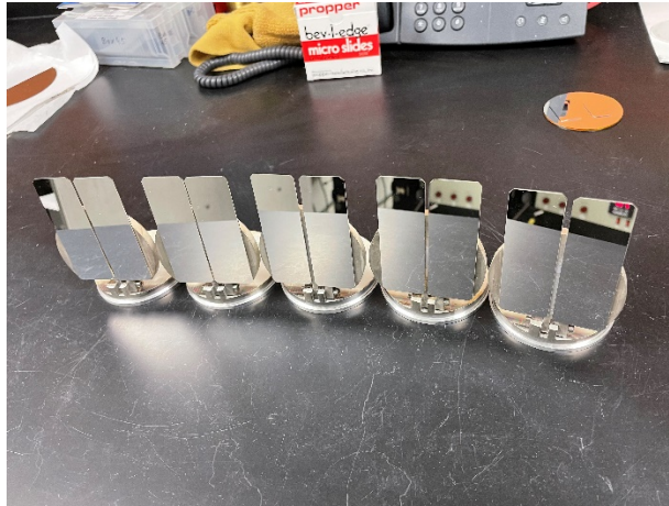
7 Fig. 6 Ag Mirror finished substrate before the GLAD deposition.
