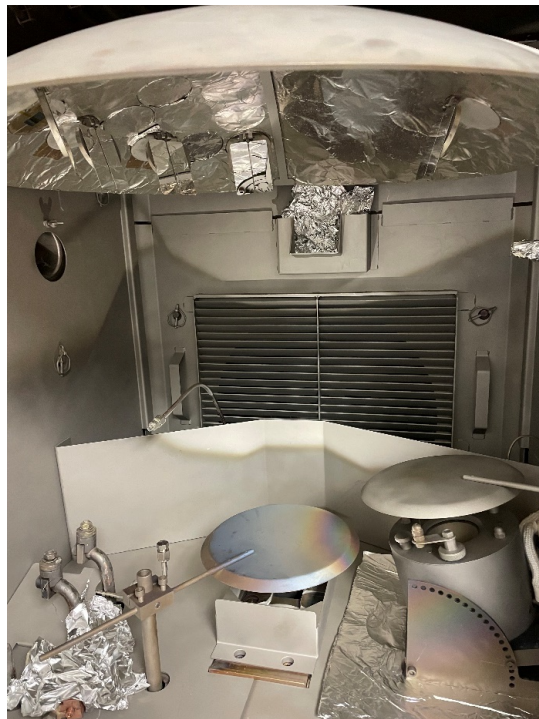
7 Fig. 6 Ag Mirror finished substrate before the GLAD deposition.
