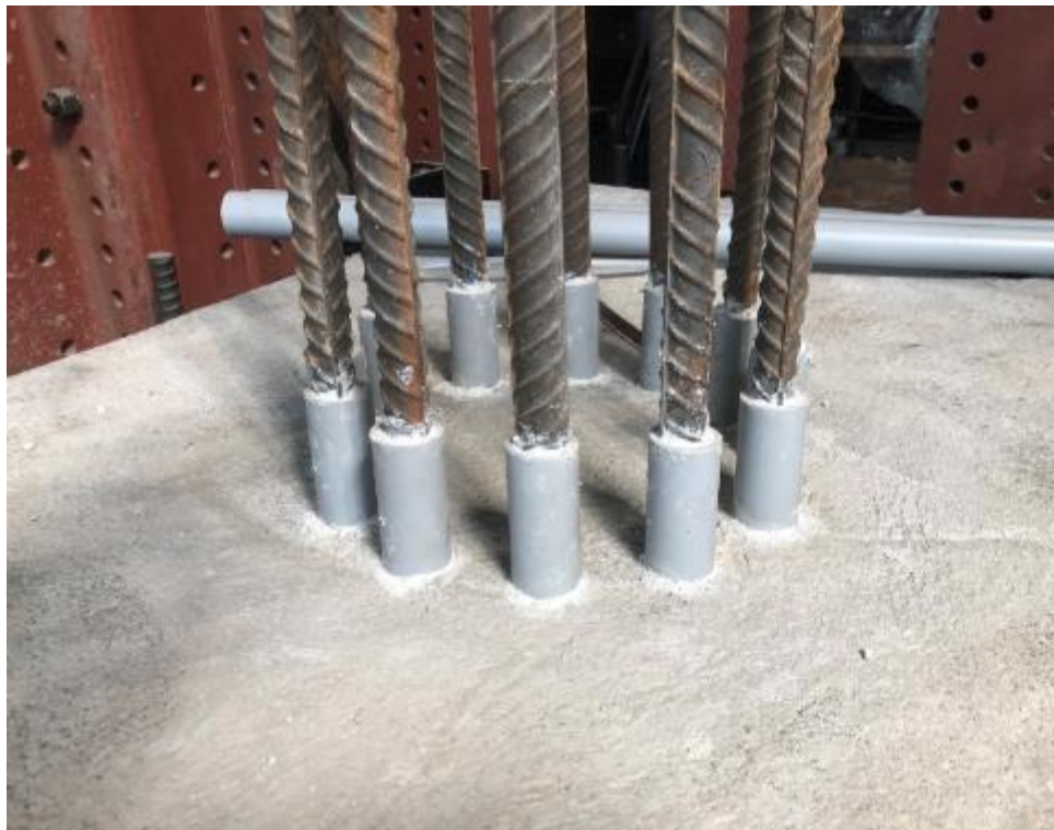
Figure 4.13 Armatures gainées (P5)
