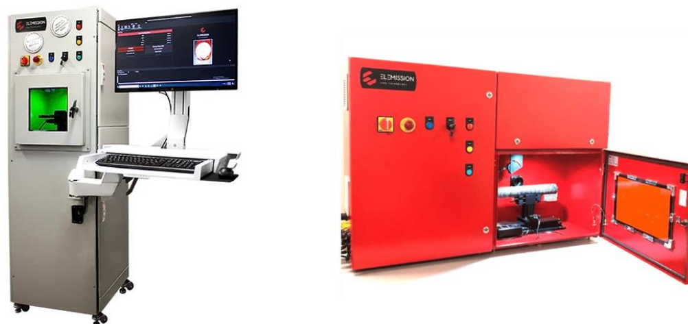
Figure 2-19 : Dispositif instrumental LIBS CORIOSITY (Elemission, 2023)
