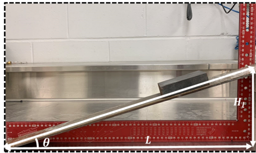
604 Fig. A5 The tilt test with a steel block and a steel plate
