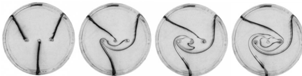
Figure 8.4 2D chaotic micromixer with 3 point-like apertures. Sequentially activating each aperture leads to a folding of the concentration pattern onto itself. Taken from [127]
