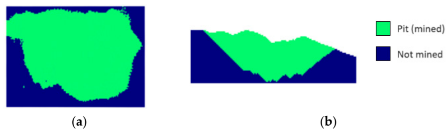
Figure 5. Stochastic final pit limit by considering a confidence level \delta = 95\% . (a) Plan view, (b) north section view—5.030 m.
