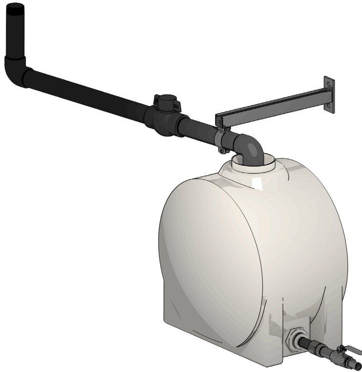
Fig. 4. 3D representation of the main tank and of its connection to the acrylic tank and to the pump.
