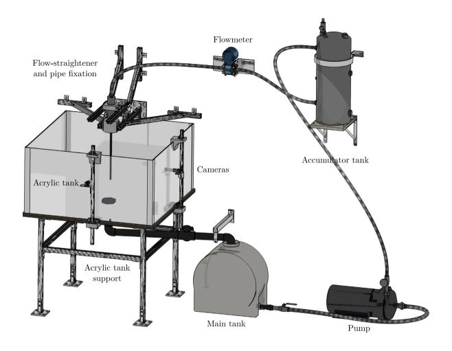
Fig. 1. 3D representation of the whole setup.
