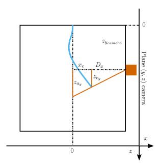
Fig. 25. Third step of parallax treatment: correction of the z height for each points.
