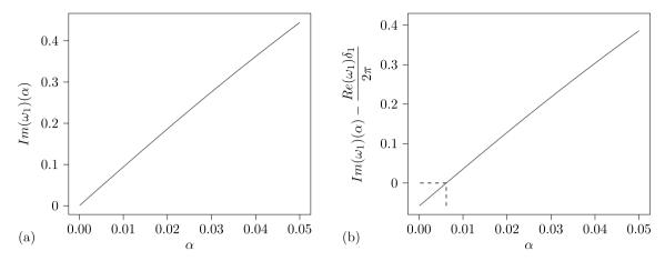
**Fig. 29.** Determination of the damping parameter  $\alpha$ : (a) Imaginary part of the first eigenvalue as a function of  $\alpha$  and (b) determination of the value of  $\alpha$  by finding the root of the function constructed with the measured frequency.
