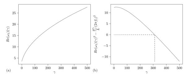
Fig. 28. Determination of the  $\gamma$  parameter: (a) Real part of the first eigenvalue as a function of  $\gamma$  and (b) determination of the value of  $\gamma$  by finding the root of the function constructed with the measured frequency.
