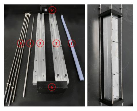
$\textbf{Fig. 3.} \ \ \textbf{Photo of the mould used to cast the pipe conveying fluid with rubber silicon.}$
