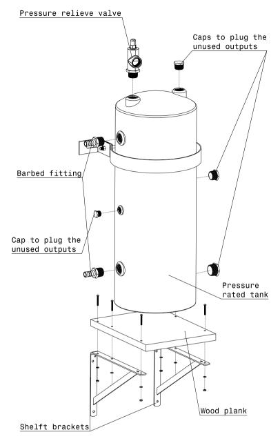
Fig. 9. Exploded view representing the assembly of the accumulator tank.
