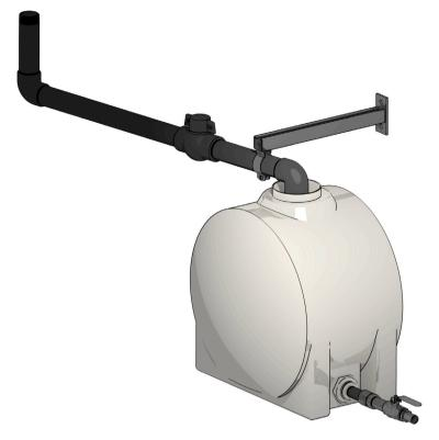
Fig. 4. 3D representation of the main tank and of its connection to the acrylic tank and to the pump.
