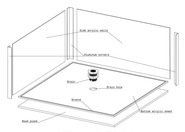
$\textbf{Fig. 15.} \ \ \textbf{Exploded view representing the assembly of the acrylic tank}.$
