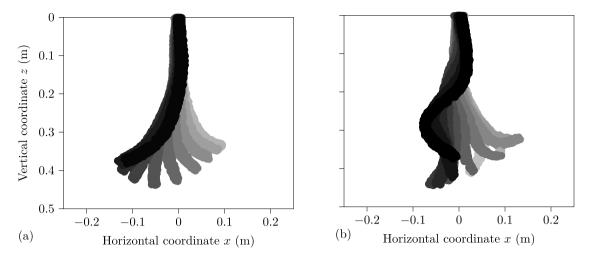
Fig. 30. Snapchots of the pipe with length 46 cm and inner diameter 6.35 mm taken every 0.02 s for different non-dimensional flowrates (a): u = 21.98, (b): u = 30.20.
