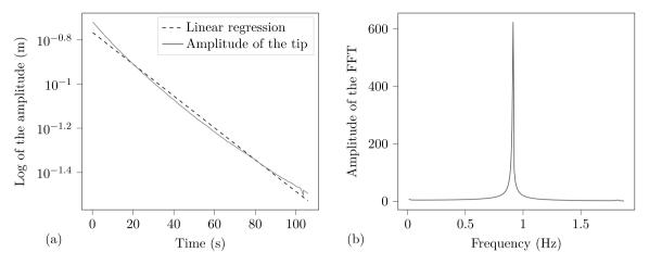
Fig. 27. (a): Comparison of the logarithmic amplitude of the tip and linear regression associated and (b) result of the FFT of the position of the tip.
