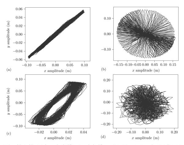
**Fig. 31.** Trace of the tip of the pipe in the (x, y) plane for different pipes and reduced flowrates: (a) d = 6.35 mm, L = 46 cm and u = 17.49, (b) d = 6.35 mm, L = 46 cm and u = 22.70, (c) d = 6.35 mm, L = 46 cm and u = 30.21 and (d) d = 9.525 mm, L = 46 cm and u = 63.95.
