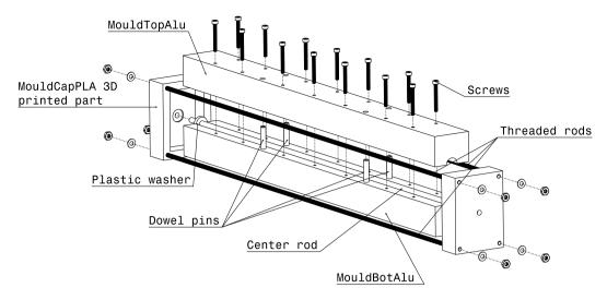
Fig. 22. Exploded view representing the mould.
