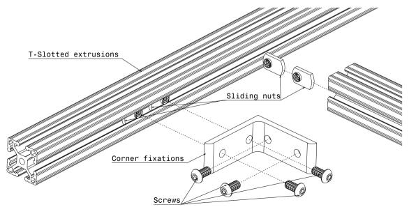
$\textbf{Fig. 17.} \ \ \textbf{Exploded view representing the assembly of two aluminium extrusions with a corner.}$
