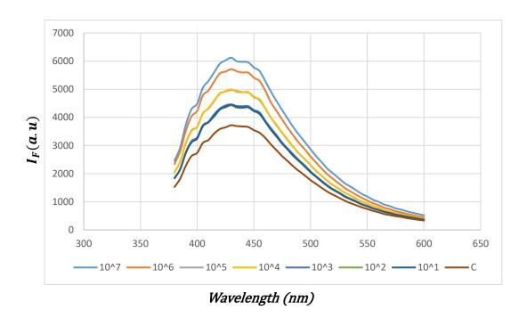
Figure 4.33 Fluorescence spectra of 4-Nitrophenyl  $\alpha$ -D-mannopyranoside-CQDs for the detection of E. coli K12 in Lemonade. Same day - Same batch
