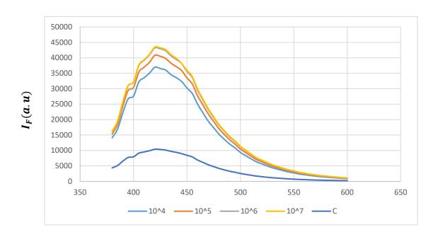
Figure 4.18 Fluorescence spectra of Man-CQDs  $(\times 1)$  for the detection of E. coli K12 in Tap Water; Different days - Same batch
