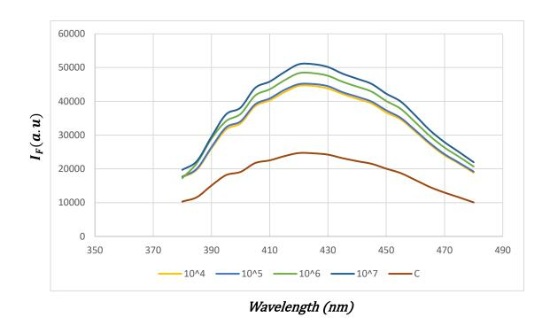
Figure 4.12 Fluorescence spectra of Man-CQDs (×1) for the detection of E. coli K12 in PBS Series two: Different days - Same batch
