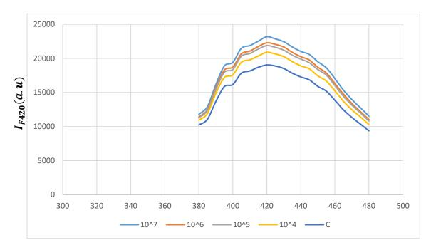
Figure 4.20 Fluorescence spectra of Man-CQDs  $(\times 1)$  for the detection of E. coli K12 in Apple Juice; Same day - Same batch
