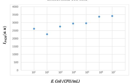
Figure 4.4 Fluorescence intensity (at 420nm) of Man-CQDs (0.1×) and E. coli K12 in PBS
