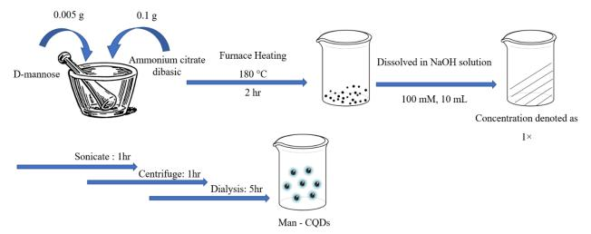
Figure 3.1 Schematic representation of the synthesis of mannose modified carbon quantum dots
