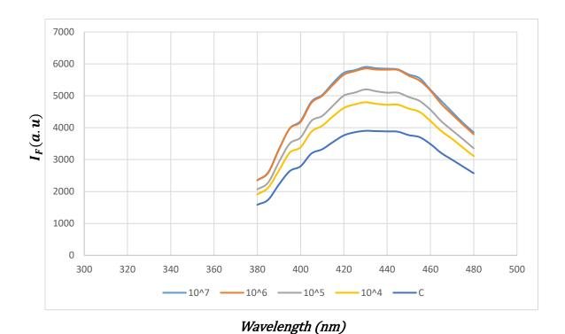
Figure 4.22 Fluorescence spectra of Man-CQDs  $(\times 1)$  for the detection of E. coli K12 in Lemonade; Same day - Same batch
