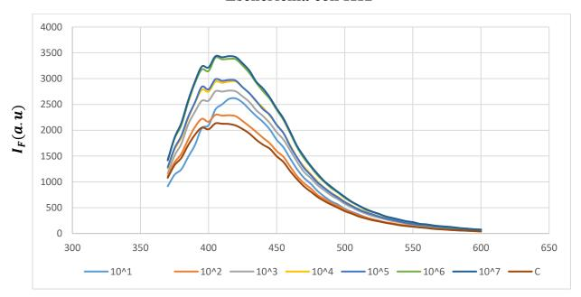
Figure 4.3 Fluorescence spectra of Man-CQDs (×0.1) for the detection of E. coli K12 in PBS
