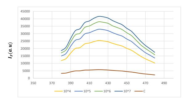
Figure 4.14 Fluorescence spectra of Man-CQDs (×1) for the detection of E. coli K12 in PBS
