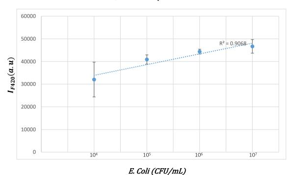
Figure 4.19 Fluorescence intensity (at 420nm) of Man-CQDs ( $1\times$ ) and E. coli K12 in Tap Water; Different days - Same batch
