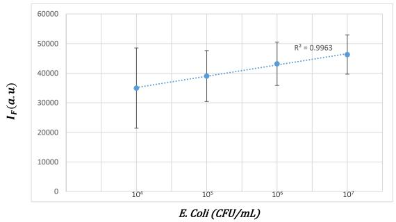
Figure 4.15 Fluorescence intensity (at 420nm) of Man-CQDs (1×) and E. coli K12 in PBS
