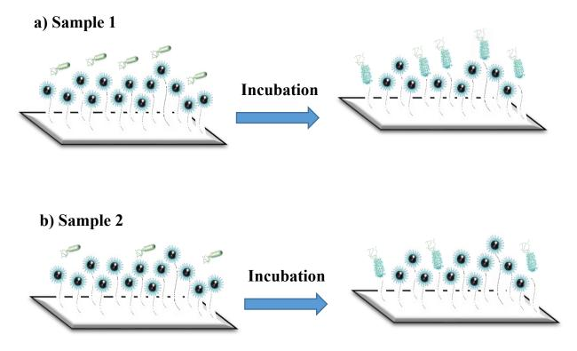
Figure 5.2 Detection mechanism in a solid-based probe a) sample 1: detection procedure for a sample containing a higher concentration of E. coli. b) sample 2: detection procedure for a sample containing a lower concentration of E. coli.
