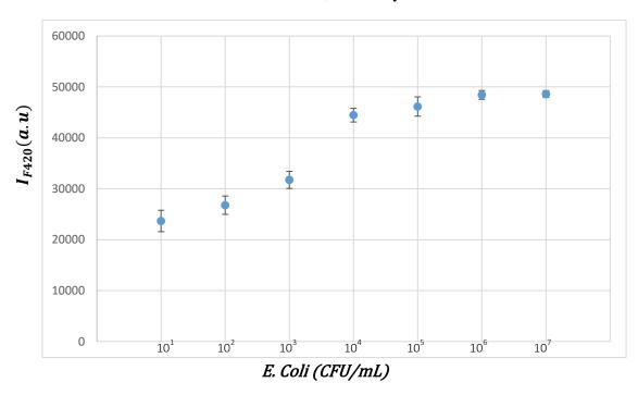
Figure 4.27 Fluorescence intensity (at 420nm) of 4-Nitrophenyl  $\alpha$ -D-mannopyranoside-CQDs and E. coli K12 in PBS; Same day - Same batch
