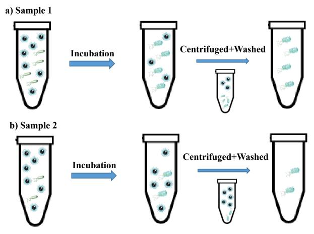
Figure 5.1 Detection mechanism in a liquid-based probe a) sample 1: detection procedure for a sample containing a higher concentration of E. coli. b) sample 2: detection procedure for a sample containing a lower concentration of E. coli.
