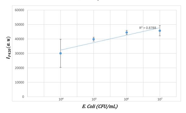
Figure 4.17 Fluorescence intensity (at 420nm) of Man-CQDs ( $1\times$ ) and E. coli K12 in Tap Water; Same day - Same batch
