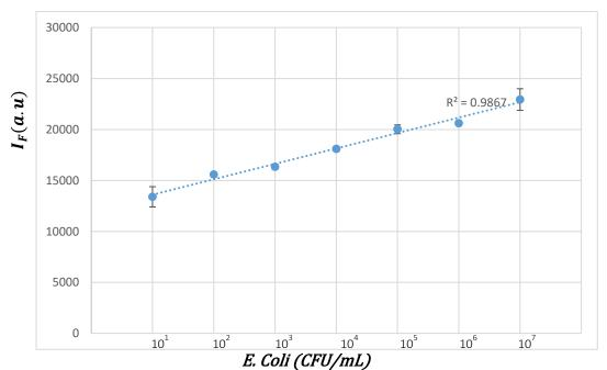
Figure 4.32 Fluorescence intensity (at 420nm) of 4-Nitrophenyl α-D-mannopyranoside-CQDs and E. coli K12 in Apple Juice. Same day - Same batch
