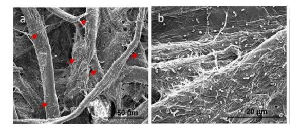
Figure 2.6 FESEM images of FimH+ cells captured on the filter paper infused with CNFs-mannose
