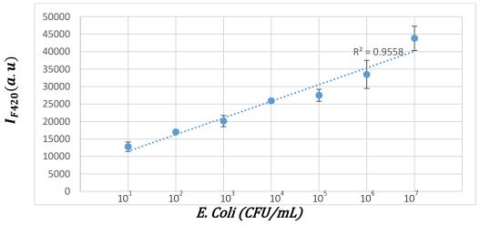
Figure 4.30 Fluorescence intensity (at 420nm) of 4-Nitrophenyl  $\alpha$ -D-mannopyranoside-CQDs and E. coli K12 in Tap Water. Same day - Same batch
