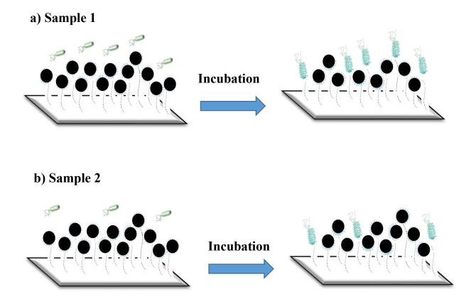
Figure 5.3 Detection mechanism in a solid-based probe with quenching mechanism a) sample 1: detection procedure for a sample containing a higher concentration of E. coli. b) sample 2: detection procedure for a sample containing a lower concentration of E. coli.
