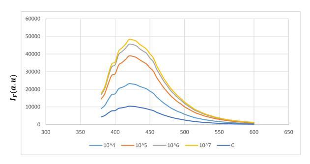
Figure 4.16 Fluorescence spectra of Man-CQDs  $(\times 1)$  for the detection of E. coli K12 in Tap Water; Same day - Same batch
