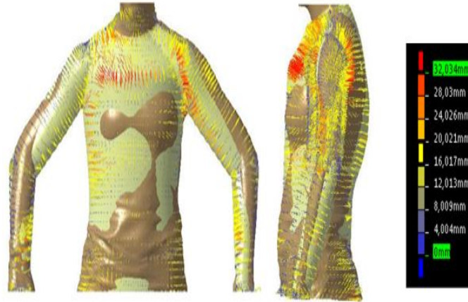
Figure 3.4 The overlapped (mm) between CAD modeled surface coverage and InSpeck non-contact laser scanner.
