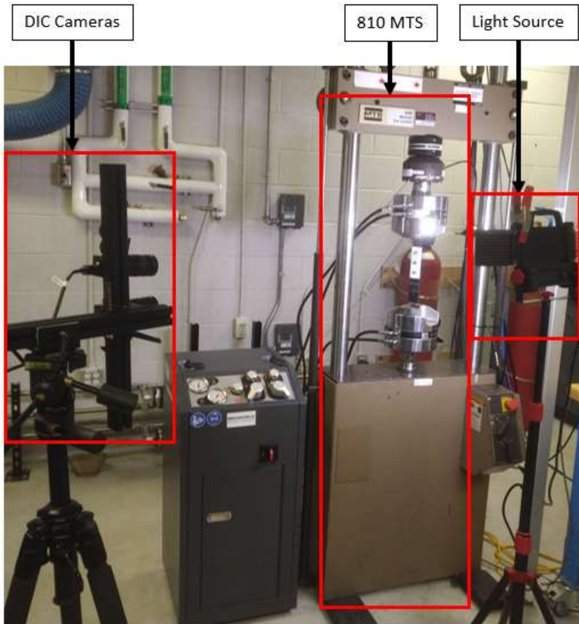
Figure 3-5: Uniaxial tensile test setup with DIC cameras
