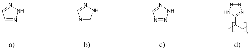
Figure 2.5 Structure of a) 1,2,3 triazole b) 1,2,4 triazole c) tetrazole d) Poly vinyl tetrazole PVT
