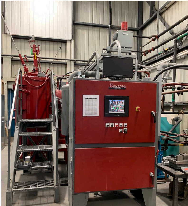
Figure 3.1 Picture of a CONSARC furnace which operates in a closed system under vacuum
