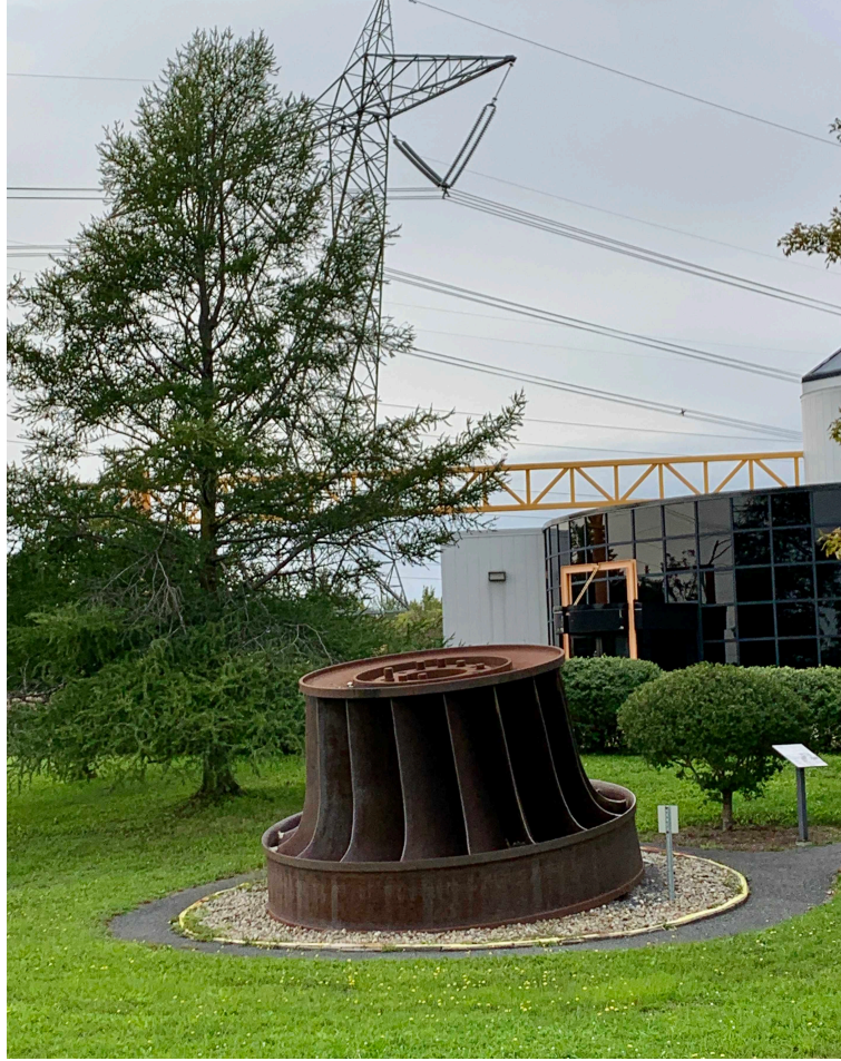
Figure 1.1 Old Francis turbine (picture taken at Hydro-Québec Électrium in Sainte-Julie, QC)
