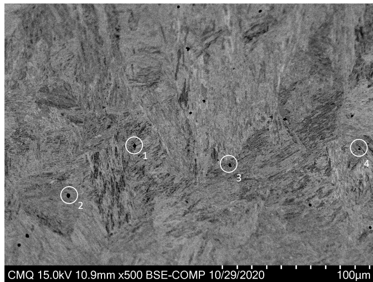
Figure 4.17 SEM image with selected inclusions from the bar 2019C-I, heat-treated condition (magnification 500x)
