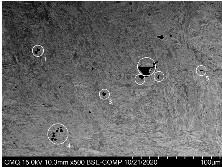
Figure 4.30 SEM image with selected inclusions from the bar 2020V-VIII, as-cast condition (magnification 500x)
