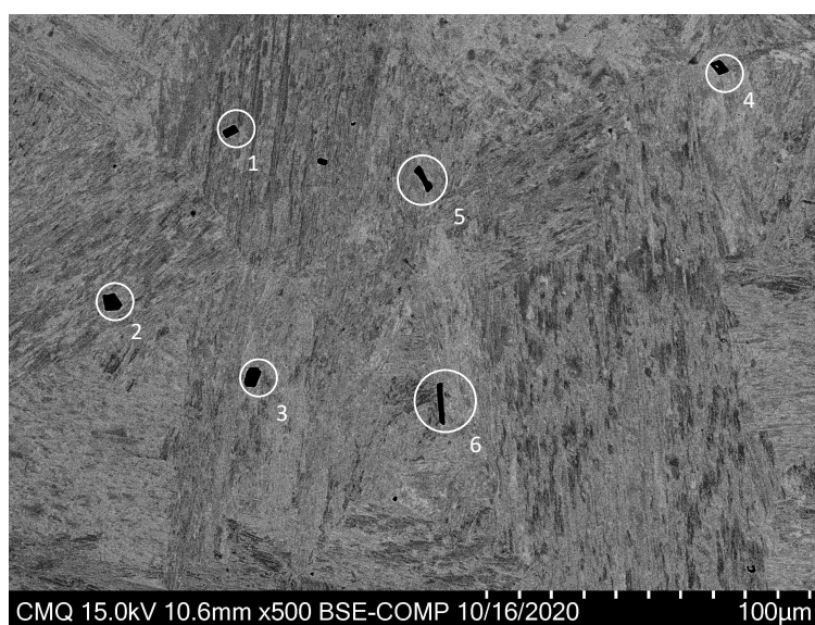
Figure 4.23 SEM image with selected inclusions from the bar 2019V-I, heat-treated condition (magnification 500x)
