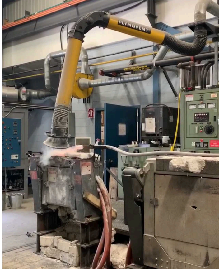
Figure 3.2 Picture of the VIP furnace during a melting process with liquid argon being poured on top of the melt
