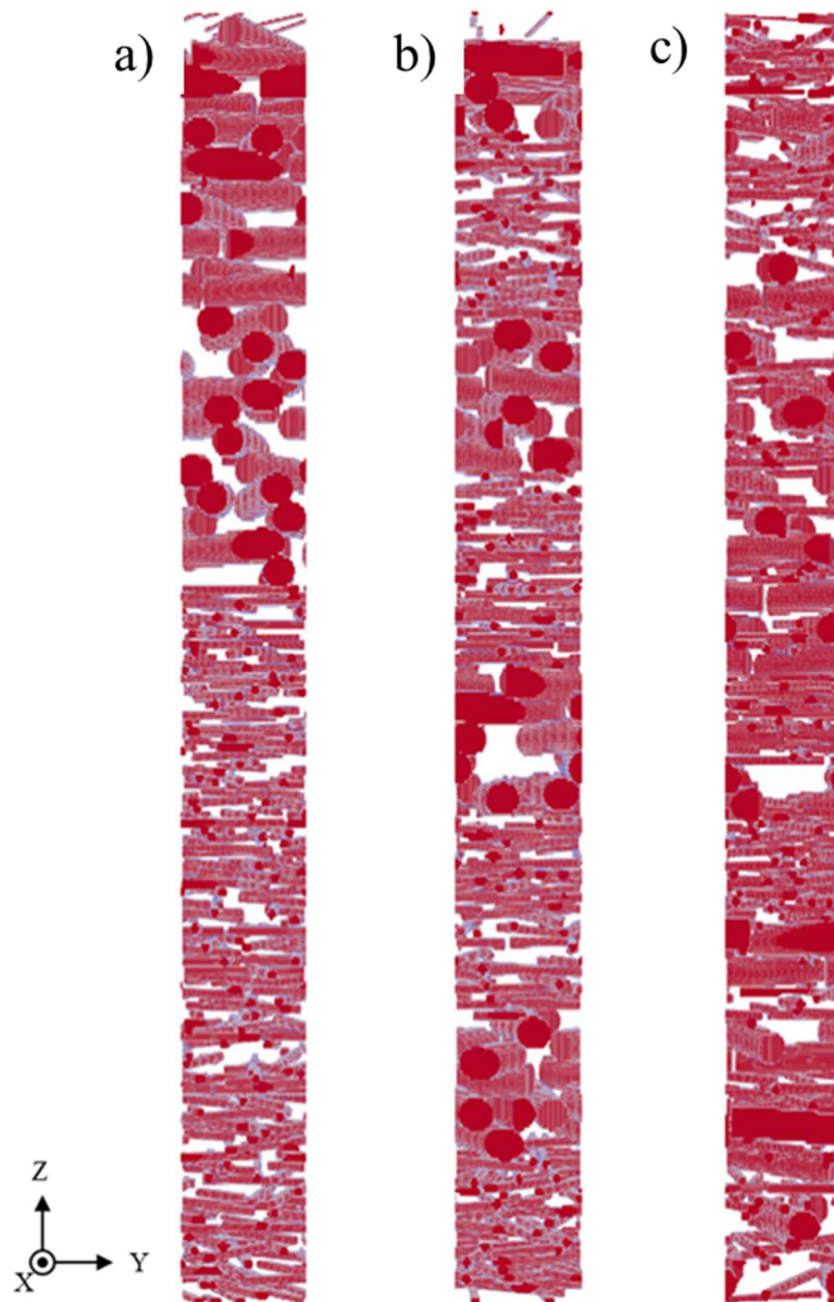
Figure 3.9 Examples of representative elementary volumes of filter media created by the fibre deposition algorithm to study the impact of multilayering for the: a), two-layered; b), eight-layered; and c), well-mixed cases, with d_C = 12 \mu m and x_F = 30\%
