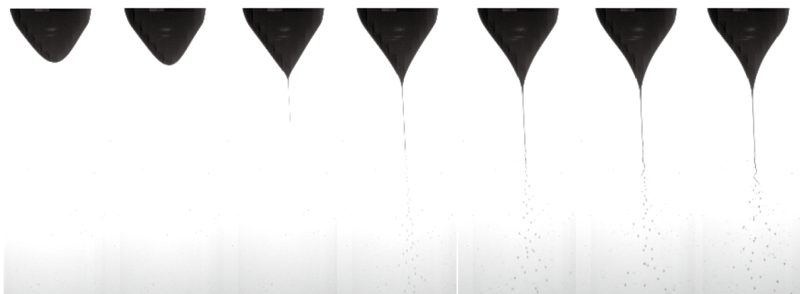
Figure 2.2 Close-up of cone-jet mode electrospraying process. From left to right it's possible to note the formation of the solution jet and its consequent break up into droplets [4].
