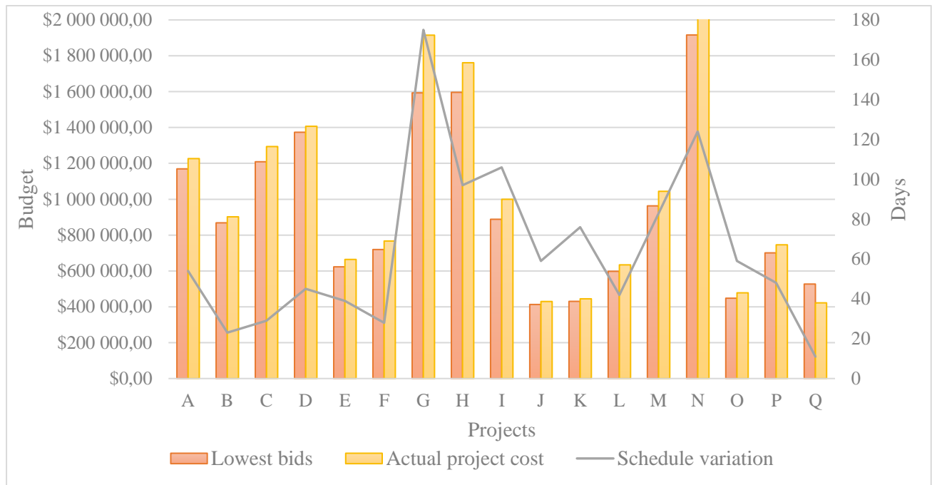
Figure 5.4 Lowest bids' impact on the schedule variation and on actual project cost
