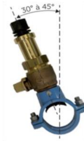
Figure 3.6 Angle of installation of the KAPTA 3000 monitoring probes
