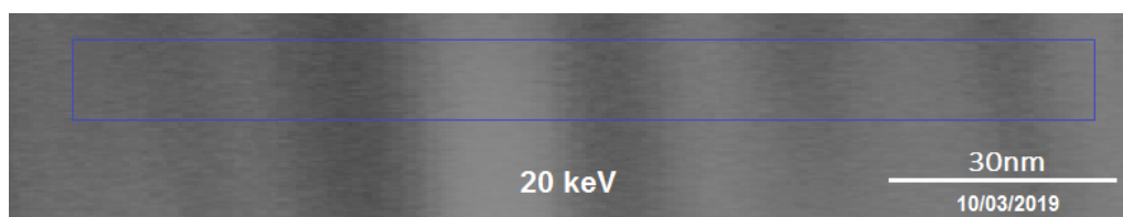
Figure 5.4 The selected region from sample S6 where the Auger Spectroscopy has been performed. The light and dark area correspond to Ni and Cu respectively.
