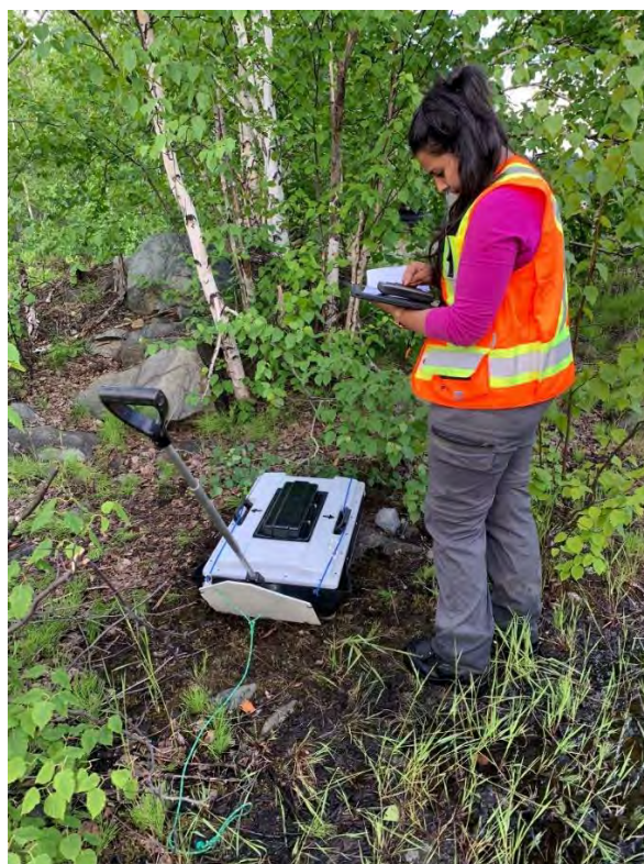
Figure 4.7 GPR Mala vision du GRES
