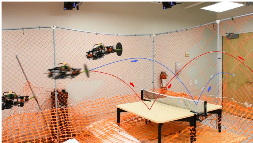
Figure 4.5. The developed quadrotor in action during a hitting motion.
