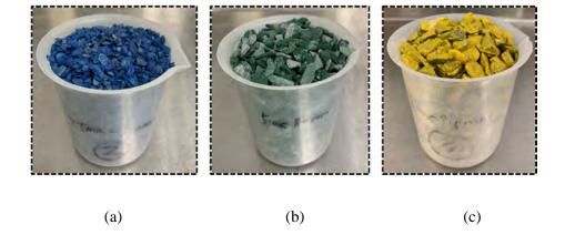
Fig. 5 Tinted waste rocks samples with different particle sizes: (a) small particle sizes in the range of 2.5
