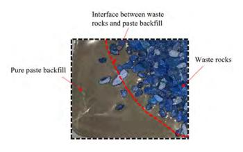
In this study, corrections were made by excluding the mass of pure paste backfill  $M'_{paste.dried}$ , estimated based on observation of pictures, as shown in Fig. A2. The solids contents by mass of waste rocks and the mixing degree of the mixture based on these corrections are presented in Table A2.
