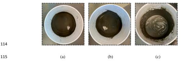
**Fig. 3** Pictures of paste backfills having solids contents by mass of: (a) 70%, (b) 72.5%, and (c) 75%, respectively
