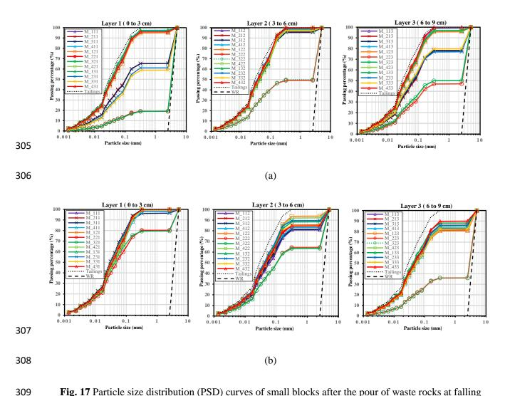
**Fig. 17** Particle size distribution (PSD) curves of small blocks after the pour of waste rocks at falling heights of: (a) 45 cm (Case 6); (b) 75 cm (Case 7)
