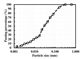
Fig. 1 Particle size distribution curve of the tested tailings
