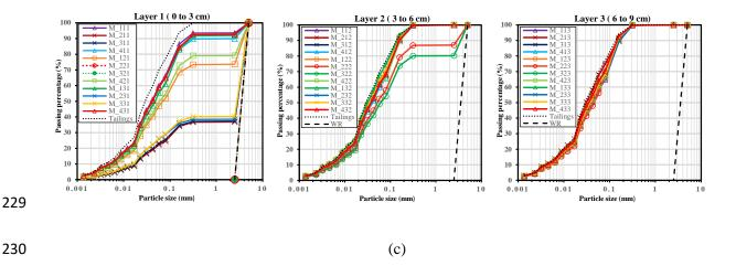
**Fig. 11** Particle size distribution (PSD) curves of small blocks after the pour of waste rocks in the paste backfills having solids contents by mass of: (a) 70% (Case 1); (b) 72.5% (Case 2); (c) 75% (Case 3)
