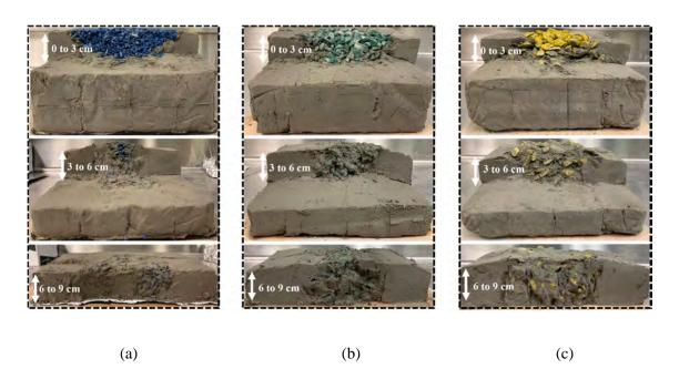
**Fig. 13** Internal structures of the mixtures after the pour of waste rocks with: (a) small particle sizes (Case 2); (b) medium particle sizes (Case 4); (c) large particle sizes (Case 5)
