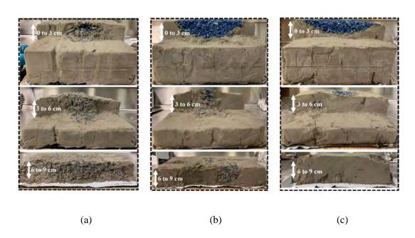
**Fig. 10** Internal structures of the mixtures after the pour of waste rocks in the paste backfills having solids contents by mass of: (a) 70% (Case 1); (b) 72.5% (Case 2); (c) 75% (Case 3)
