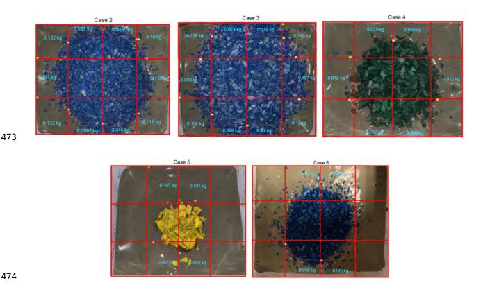
Fig. A2 Estimation of the mass of pure paste backfill in each block at layer 1
