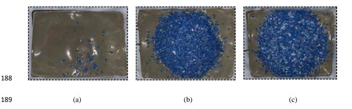
**Fig. 9** Top views of the mixtures after the pour of waste rocks in the paste backfills having solids contents by mass of: (a) 70% (Case 1); (b) 72.5% (Case 2); (c) 75% (Case 3)
