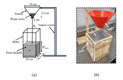
**Fig. 6** A physical model to study the natural mixing behavior of waste rocks poured in a paste backfill: (a) schematic presentation; (b) a picture
