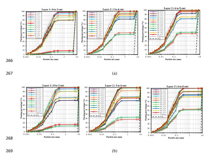
**Fig. 14** Particle size distribution (PSD) curves of small blocks after the pour of waste rocks with: (a) medium particle sizes of 5.0 to 8.0 mm (Case 4); (b) large particle sizes of 8.0 to 9.5 mm (Case 5)
