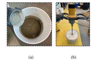
**Fig. 2** Procedures for making a homogenous paste backfill: (a) addition of dried tailings into water; (b) mixing with an electric stirring rod
