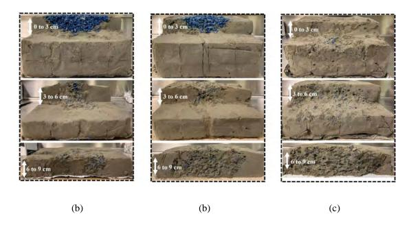
**Fig. 16** Internal structures of the mixtures after the pour of waste rocks at falling heights of: (a) 15 cm (Case 2); (b) 45 cm (Case 6); (c) 75 cm (Case 7)
