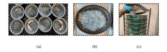
**Fig. 8** Procedure for obtaining the particle size distribution curves of a small block: (a) small blocks after 24 hours of oven-drying; (b) hand-crushed mixture of a dried block; (c) sieving analysis
