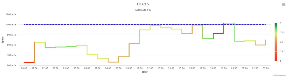
Figure 5.5 Using color on a step line as a data uncertainty visualization technique
