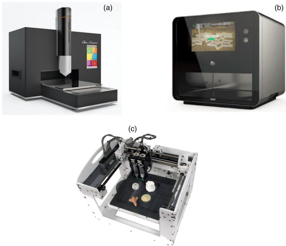
Figure 2.1 Three examples of existing commercial extrusion-based 3D food printers [38]: a) Choc Creator (Choc Edge, 2018) [39], b) Foodini (Natural Machines, 2020) [40] and c) Fab@Home (Creative Machines, 2020 [41]).
