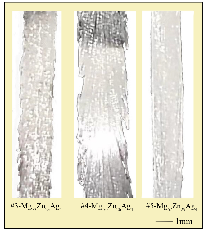
Fig. 3. The images of the Mg-Zn-Ag metallic glasses with the #3- \text{Mg}_{73}\text{Zn}_{23}\text{Ag}_4 , #4- \text{Mg}_{70}\text{Zn}_{26}\text{Ag}_4 and #5- \text{Mg}_{67}\text{Zn}_{29}\text{Ag}_4 compositions.
