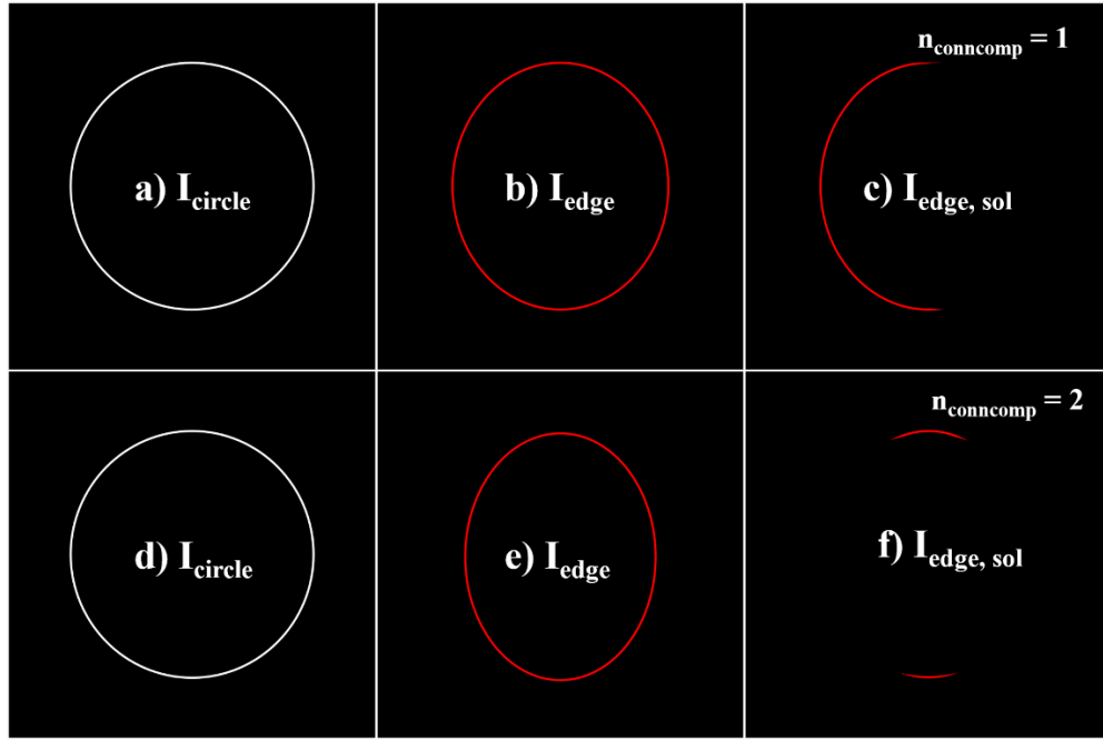
Figure 5.8: Illustration of the operations leading to the quantification of the edge fragmentation matching with a solution point for an edge with low fragmentation (images a, b, c) and high (images d, e, f) fragmentation
