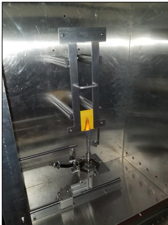
Figure 4.12: Federal Aviation Administration (FAA) flame spread test cabinet showing the piloted ignition of a sample material using a Bunsen flame, applied for 12 or 60 seconds in the vertical orientation.
