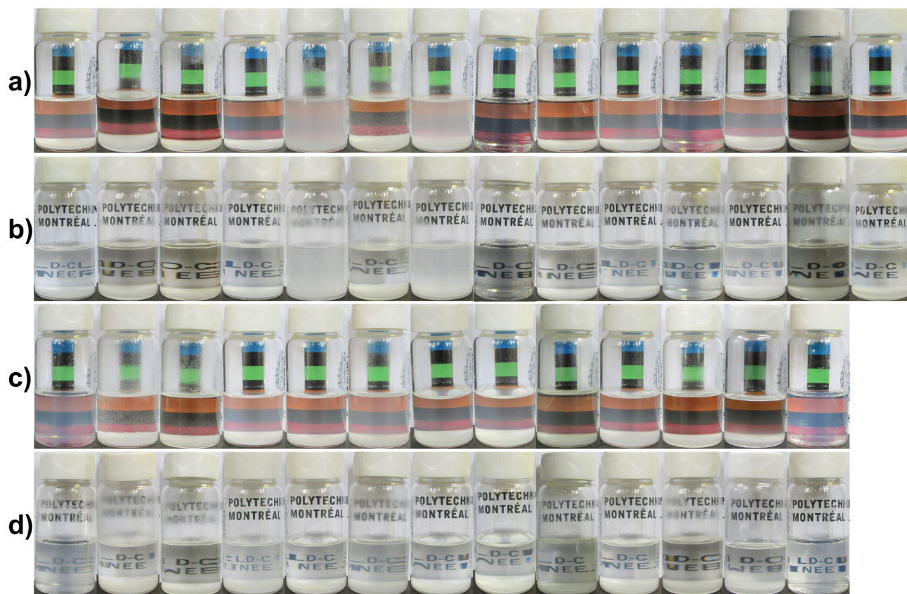
Figure B.1 Sedimentation tests in the set of pure solvents: pictures of the vials were taken after a relative sedimentation time ( RST ) of 11.8 \times 10^{11} \text{ s}^2\text{m}^{-2} on 2 different backgrounds: a colorful one ( a&c ), and a text ( b&d ). The only exception being triethanolamine, for which the sedimentation test was interrupted after t_{\text{sed}}=5540 \text{ h} , corresponding to a RST of 1.59 \times 10^{10} \text{ s}^2\text{m}^{-2} (13.5 % of the standard RST ), because the sedimentation was already finished. Solvents are from left to right in ( a&b ): acetone (0), benzene (0), benzyl alcohol (0), 2-butanol (0), chloroform (1), cyclohexane (0), dichloromethane (1), dimethyl sulfoxide (2), 1,4-dioxane (0), ethanol (0), ethanolamine (2), ethyl acetate (0), ethyl benzoate (0) and ethylene glycol (0). And in ( c&d ): formamide (2), heptane (0), d-limonene (0), methanol (0), methyl ethyl ketone (0), N,N-dimethyl formamide (0), 1-propanol (0), 2-propanol (0), propylene carbonate (0), tetrahydrofuran (0), toluene (0), triethanolamine (0), and water (2). Values between parenthesis correspond to their respective grades, from 0 to 2, and are summarized in Table B.1.
