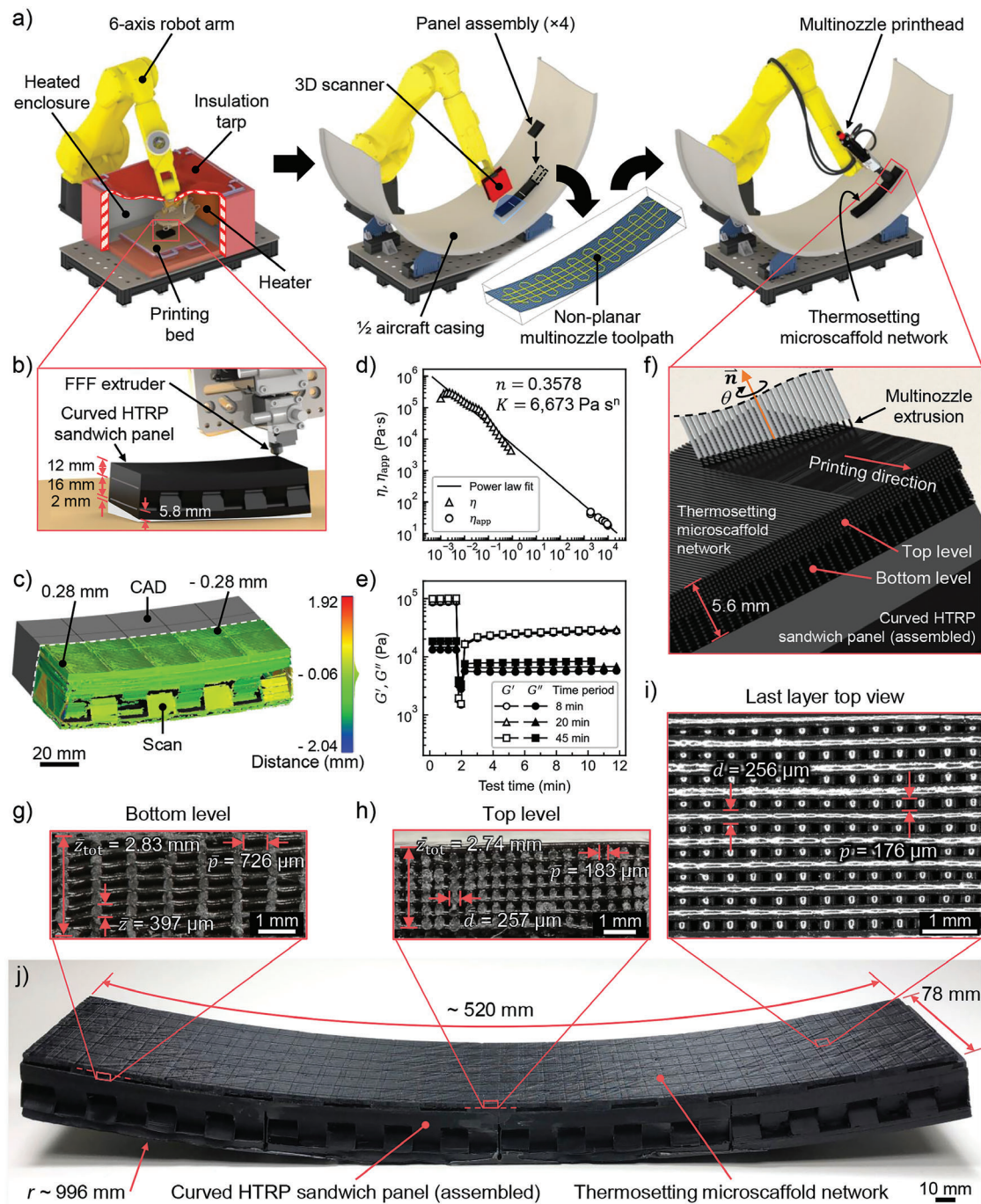
Figure 1. Non-planar multiprocess FFF of an HTRP sandwich panel and multinozzle DIW of a thermosetting microsccaffold network. a) 1) FFF of curved HTRP sandwich panel using custom heated enclosure and 6-axis robot arm (the enclosure is shown with an open cross-section to see the interior), 2) HTRP sandwich panel assembly on the aircraft casing, 3D scanning of the top surface topography, and multinozzle toolpath generation, 3) non-planar multinozzle AM of abradable thermosetting microsccaffold networks on top of HTRP panel assembly. b) Close-up view of FFF process and characteristics of a printed HTRP sandwich panel section, whose total thickness varies from 30 to 33.8 mm. c) Euclidean distance analysis from the comparison between CAD and scan mesh of a panel section. Max absolute error on top surface is 0.28 mm. d) Abradable material (OGM12FS formulation) shear-thinning behavior of viscosity \eta (obtained by rotational rheology) and process-related apparent viscosity \eta_{app} (obtained by capillary rheology). e) Shear storage G' and shear loss moduli G'' time-dependency of the abradable material (OGM12FS formulation) obtained from three interval thixotropy test (3iTT). f) Close-up view of multinozzle DIW process and characteristics of the printed microsccaffold network, whose thickness is 5.6 mm. g) Side view on the bottom porosity level, whose thickness \bar{z}_{tot} is 2.83 mm and pore size \bar{p} is 726 \mu\text{m} . h) Side view on the top porosity level, whose \bar{z}_{tot} is 2.74 mm and \bar{p} is 183 \mu\text{m} . i) Top view on the last printed layer, where \bar{d} = 256 \mu\text{m} and \bar{p} = 176 \mu\text{m} . j) Overall view of the aircraft component demonstrator. Largest radius r \approx 996 \text{ mm} , dimensions of the thermosetting microsccaffold network is \approx 520 \text{ mm} \times 78 \text{ mm} . Overall filament diameter \bar{d} = 257 \mu\text{m} and layer stacking distance \bar{z} = 397 \mu\text{m} .
