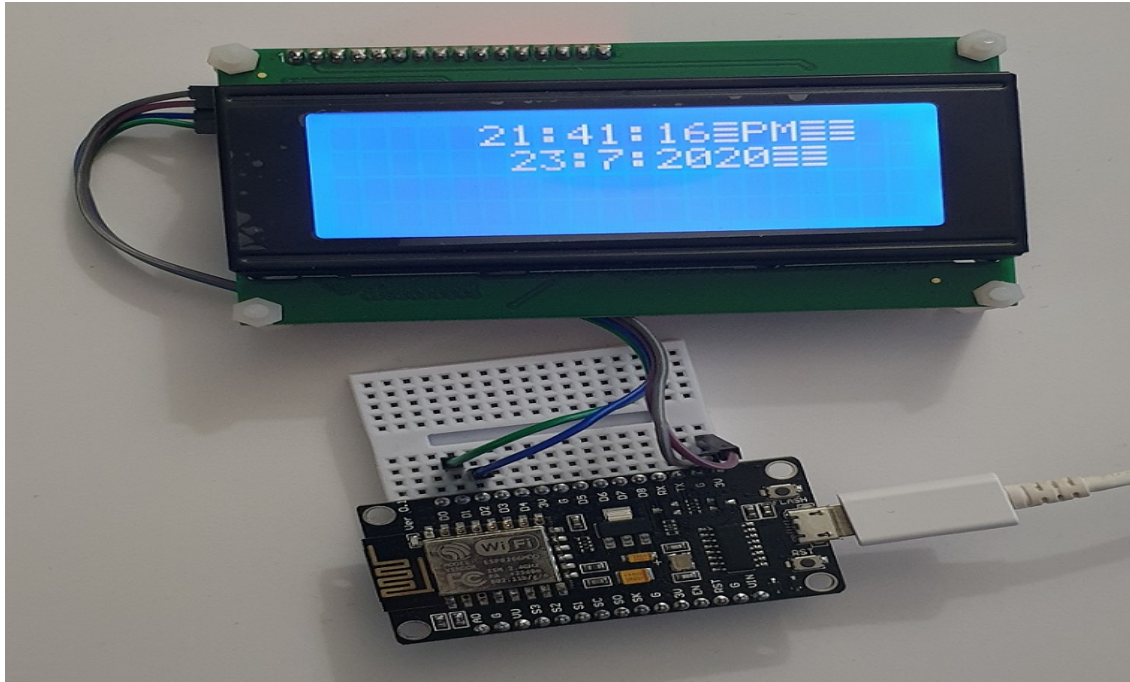
Figure 4.7 Arduino IoT LCD clock
