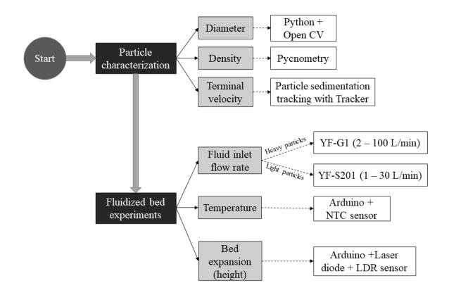
Figure 3. Workflow of the experimental procedure.
