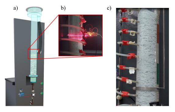
Figure 2. Schematic representation of a) the experimental setup, b) the laser apparatus, and c) the fluidization experiment.
