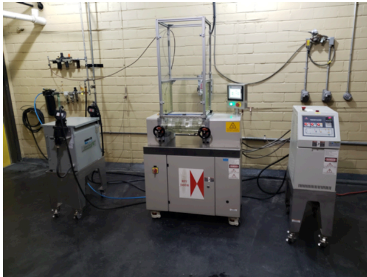
Figure 3-2 Two-roll mills equipped with a security guard (center), power supply (left) and recirculatory heater (right).
