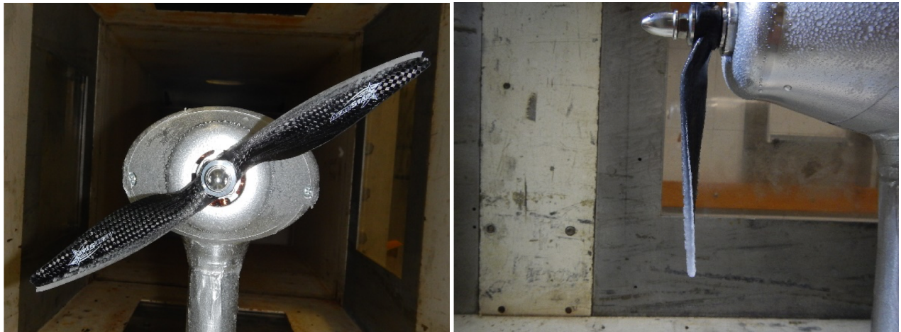
Figure 1.1 Icing on a carbon fiber propeller. Courtesy of the National Research Council Canada, Aerodynamics Laboratory & Transport Canada, RPAS Task Force Engineering
