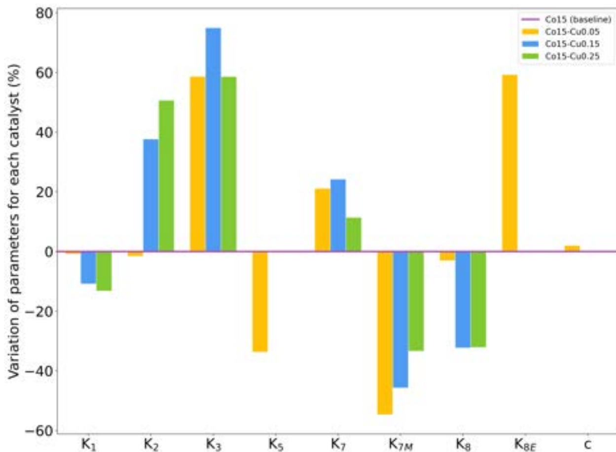
Figure 4.14 Variation of reaction kinetic parameters compared to Co15 for each of the catalysts
