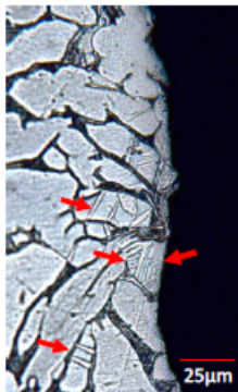
Figure 6. Twinning formations are shown by arrows under the ground surface at YZ plane
