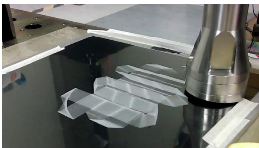
Video 4.2. Case study #2: Multinozzle additive manufacturing of a 2-layer variable pore size micro scaffold network ( 3 \times 5 configuration) at 50 \text{ mm/s} (available at https://youtu.be/xB34lHwUsog ).
