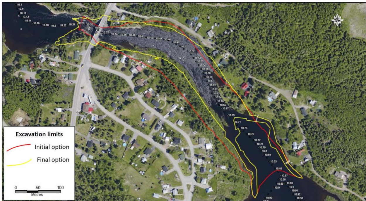
Figure 6-6 Excavation limits from the Pibrac Bridge: yellow limits correspond to option replacing the bridge with a longer one with no pillar (Modified after GENIVAR, 2009)
