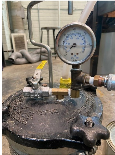
Figure A.2: Vacuum gauge and the pressure on it before doing the infusion process
