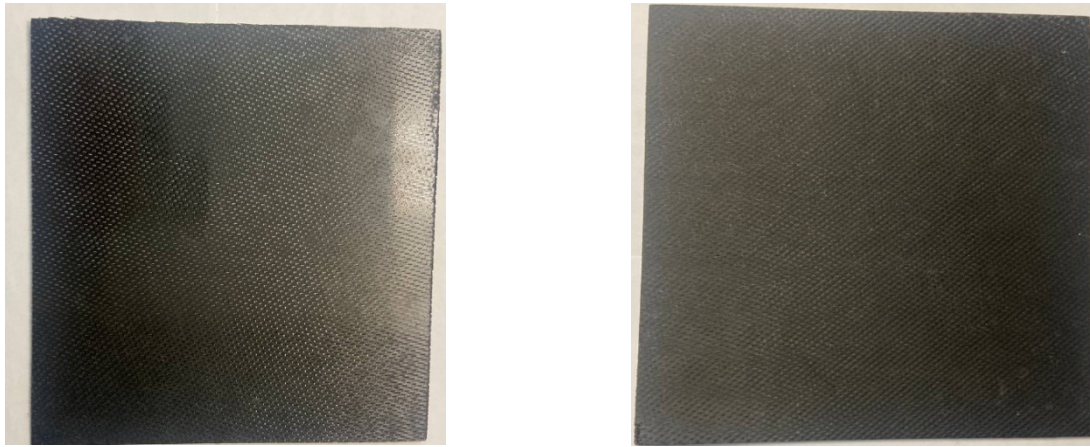
Figure 4.6: Manufactured 8-ply plate from recycled carbon fibers by V.A.R.I. method
