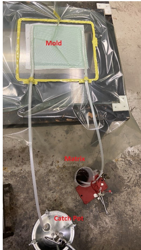
Figure A.4: V.A.R.I. method and the parts used in the process
