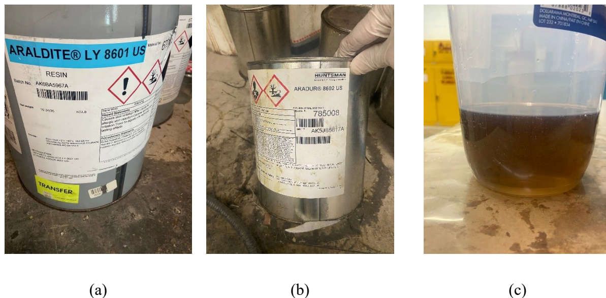
Figure 3.6: a) Resin, b) hardener and c) mixture of resin and hardener used for making matrix
