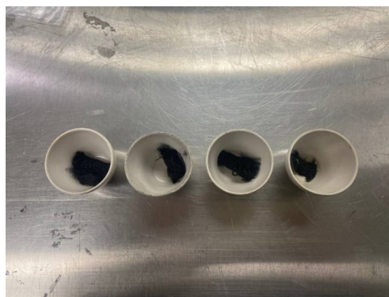
Figure 4.2- Samples after pyrolysis under 600°C
