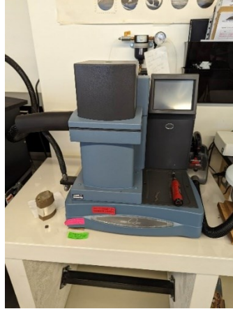
Figure 4.7: Q800 DMA used for determining T_g of the manufactured plates
