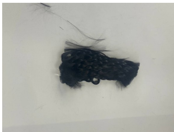
Figure 4.2- Samples after pyrolysis under 600°C
