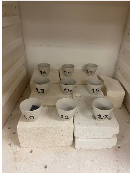
Figure 3.3: Placement of crucibles inside the furnace for pyrolysis
