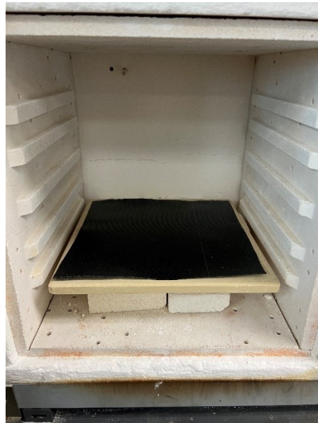
Figure 3.4: Positioning of 10" x 10" samples inside pyrolysis oven
