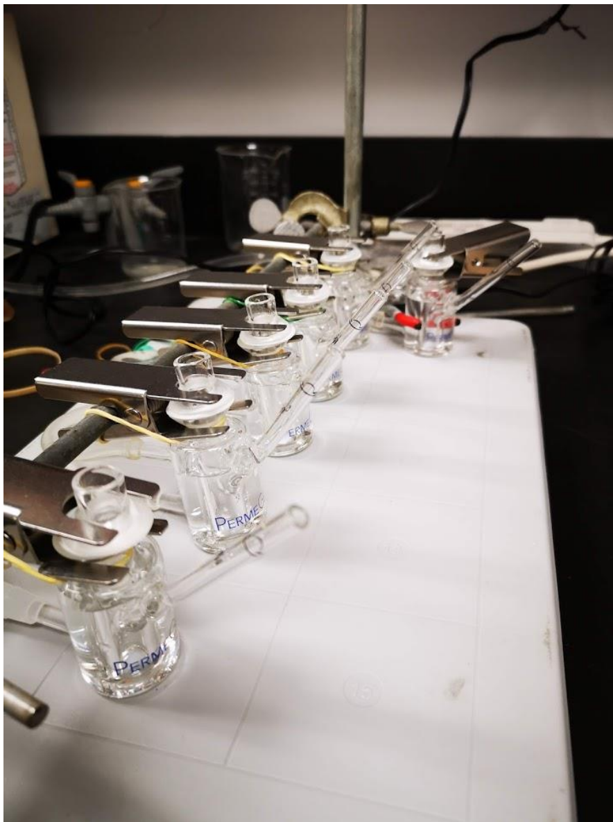
Figure 3. Franz cells in magnetic stirrer arrangement
