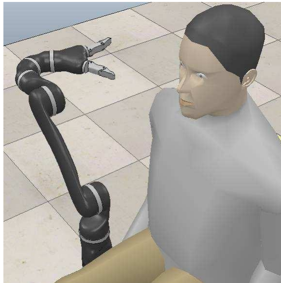
Figure 4.14 4-DOF MICO robot with gripper
