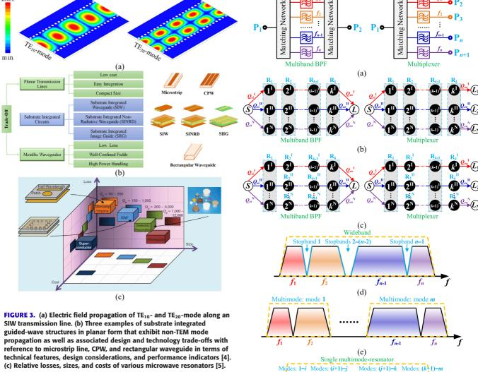
multiband BPFs and multiplexers [5]. It should be reiterated from Fig. 3(c) that SIW gathers the complementary advantages of both planar microstrip/stripline technologies and non-planar waveguide and dielectric technologies with respect to cost, size, loss, power, and processing techniques.
