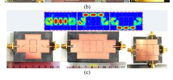
FIGURE 11. SIW multiband BPFs and multiplexers using multimodeshunting hybrid scheme. (a) Dual-band BPFs. (b) Diplexers. (c) Triple-band BPFs and triplexers.
