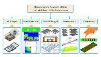
FIGURE 18. Miniaturization schemes of SIW guided-wave structures as well as SIW multiband BPFs and multiplexers.
