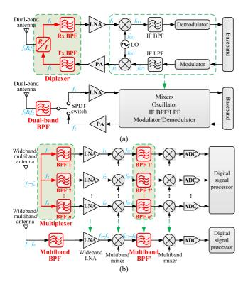
FIGURE 2. Wireless system architectures for radio communication links or radar sensing networks using multiband BPFs and multiplexers.
