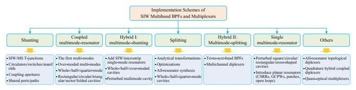
FIGURE 5. General overview of technical approaches and design highlights of SIW multiband BPFs and multiplexers.
