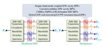
FIGURE 6. Illustration of technical approaches for developing SIW multiband BPFs and multiplexers using shunting scheme.
