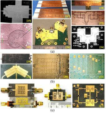
FIGURE 7. SIW T-junction-based SIW multiband BPFs and multiplexers using shunting scheme. (a) Diplexers. (b) Multiplexers based on circulator, manifold, and T-junctions. (c) CSRRs-loaded techniques.
