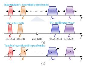
FIGURE 17. Future research and development orientations of SIW multiband BPFs and multiplexers. (a) Independent/flexible controllability of multiple channels. (b) Tunability/reconfigurability of multiple passbands.
