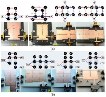
FIGURE 13. SIW multiband BPFs and multiplexers using multimodesplitting hybrid scheme. (a) Tri-/quad-/quint-band BPFs. (b) Tri-/quad-channel diplexers.
