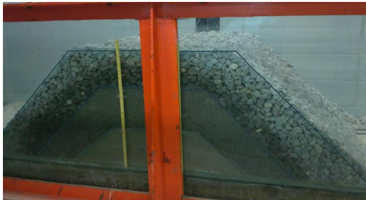
Figure 4: Marks on the glass walls of the channel of the dimensions of the layers
