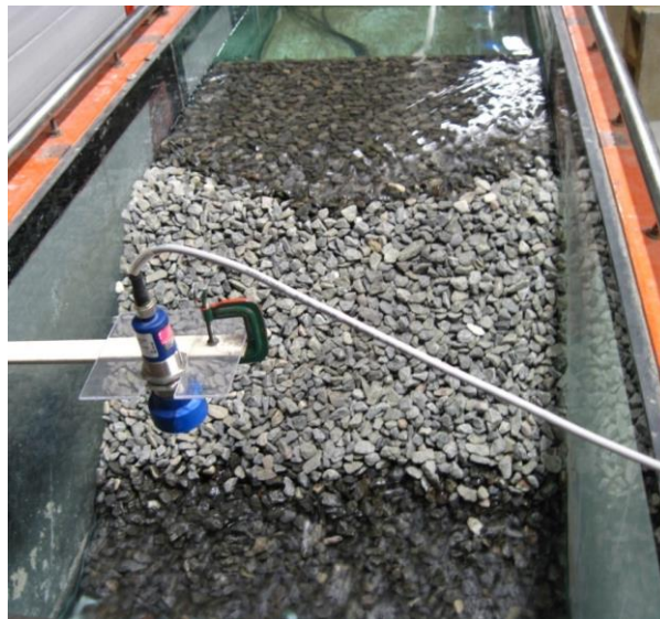
Figure 5: Phase beginning the breach at the foot of the downstream face
