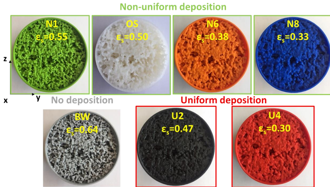
Figure 7.10: Images of the seven magnified 3D-printed twins identified by their respective sample ID (see Table 7.2) and corresponding porosity.
