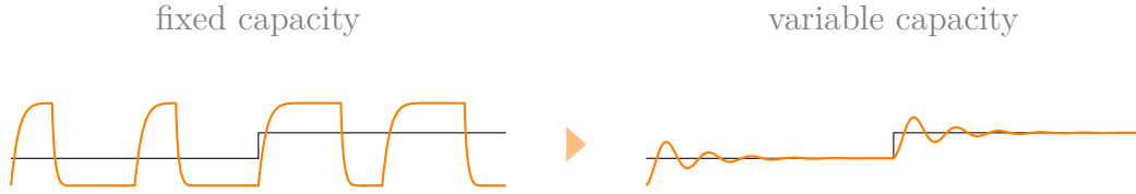
Figure 1.4: A fixed capacity heat pump must adjust the time during which it is turned on to adapt to a change in the load. On the other hand, a variable capacity heat pump can set its capacity to be exactly equal to the load.
