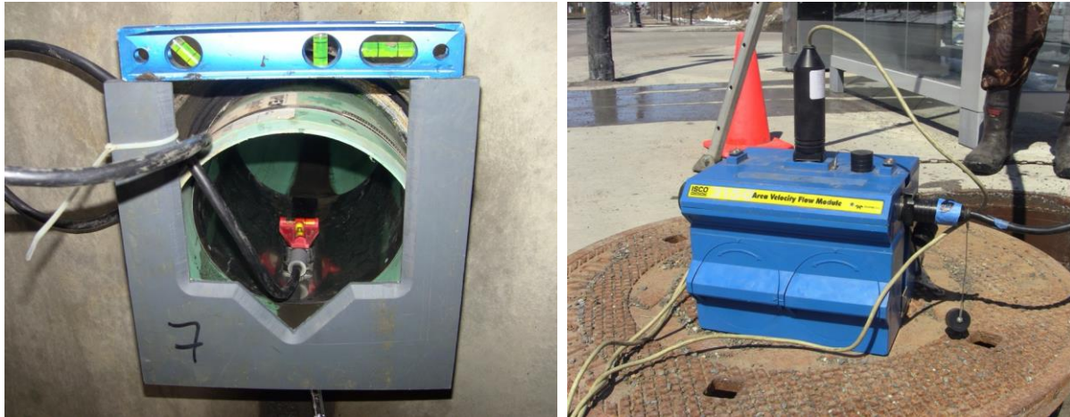
Figure 5.4 Compound weir and flowmeter installed on the downstream end of the conduit connecting a monitored point to the sewer (inside an IAW)
