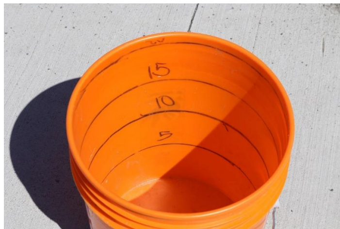
Figure B.9 Volume increments identified in a bucket used to established flow rates
