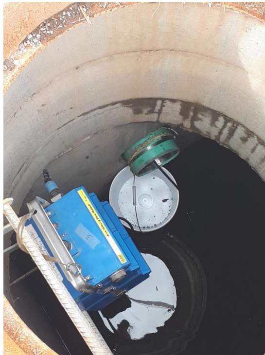
Figure 4.8 Set-up of a Teledyne ISCO 2150-Area-Velocity flowmeter inside a monitoring manhole
