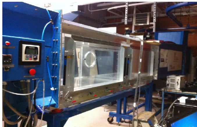
Figure 4.3 The closed-loop wind tunnel of the Fluid-Structure Interaction laboratory. The test section is shown at the center of the image.
