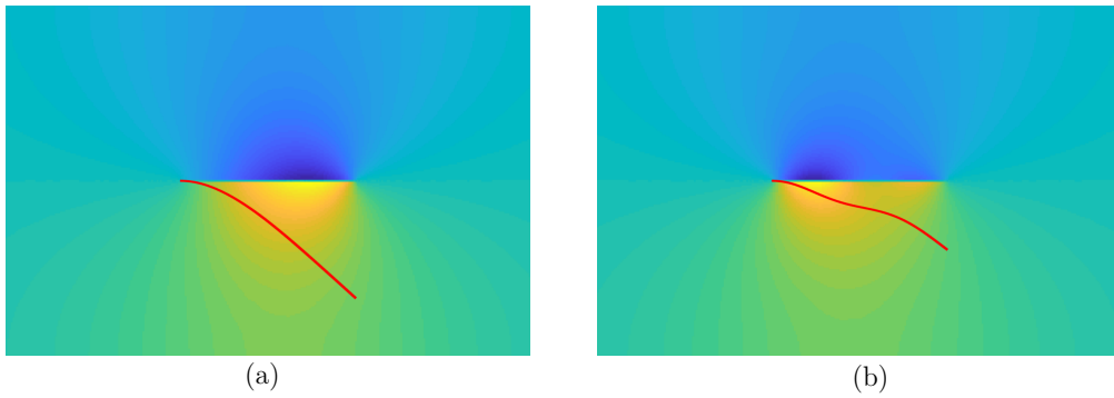
Figure 2.9 Mode shape representation for a plate with fixed-fixed boundary conditions. (a): 1st mode in a fluid at rest, (b): 1st mode with a reduced speed of U_R = 10 where the first mode is unstable.
