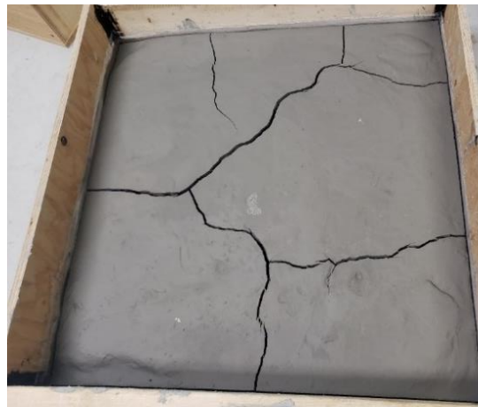
Figure 3-10: Photograph of the tailings slurry in Mold 1 with the formation of cracks on the top surface at the end of the tests.
