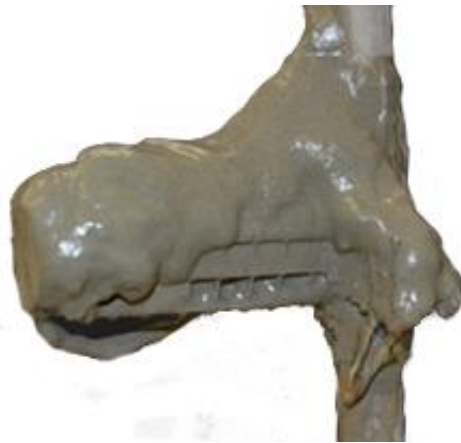
Figure 5.11 Accumulation of denser backfill on the cages and top face of the vertical stress sensor near the center of the column.
